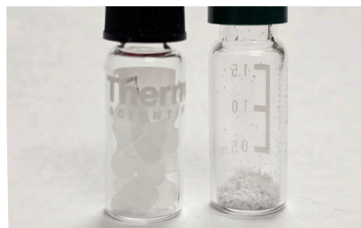
Figure 5: Polyethylene powder color comparison after conditioning the sample jar (left: original Polyethylene pellets, right: powder after grinding)
